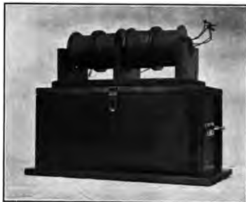
PLATE II. — Transformer for 12" Apparatus.
