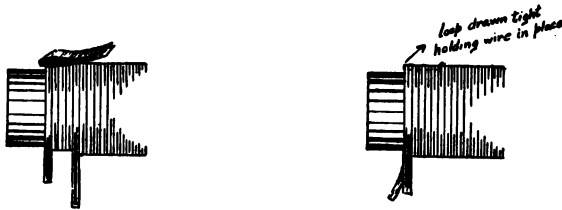
Diagrams showing manner of fastening last turn.
