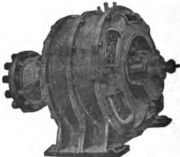
FIG. 169.—BROWN'S TWO-PHASE MOTOR OF 120 HORSE-POWER.
