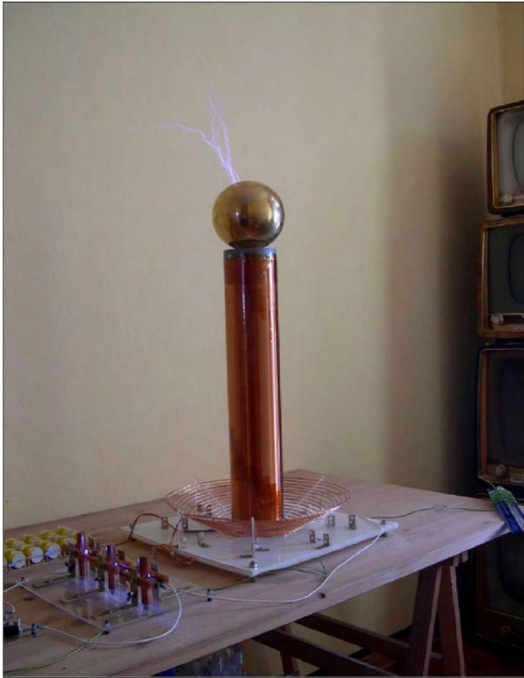
Streamers are formed even without a field-amplifying piece of wire, but their discharge strength varies greatly.
