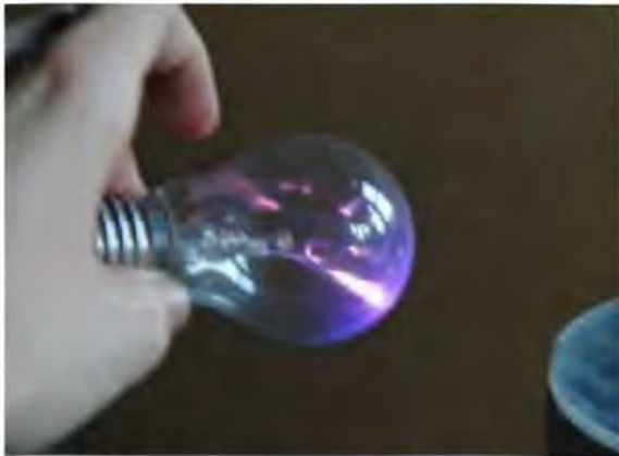
Figure 13: Plasma discharge in a light bulb without sparkover to the tesla transformer
