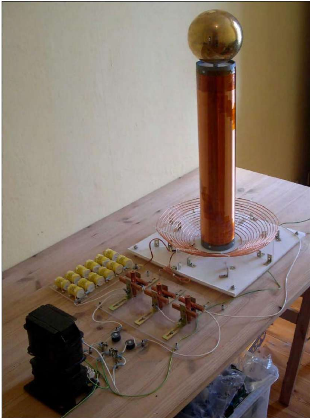
The overall structure of the Teslatrafo.
