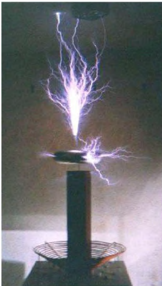
Fig. 8: Peak discharges with the aid of a piece of wire
