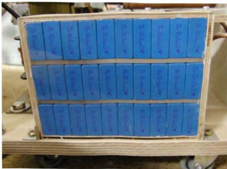
Figure 8: MMC, 10 pieces in series (string), three strings parallel
