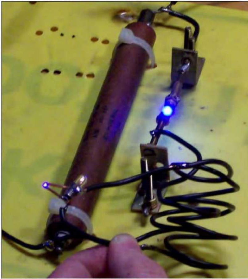
The sparkover parallel to the bulb
