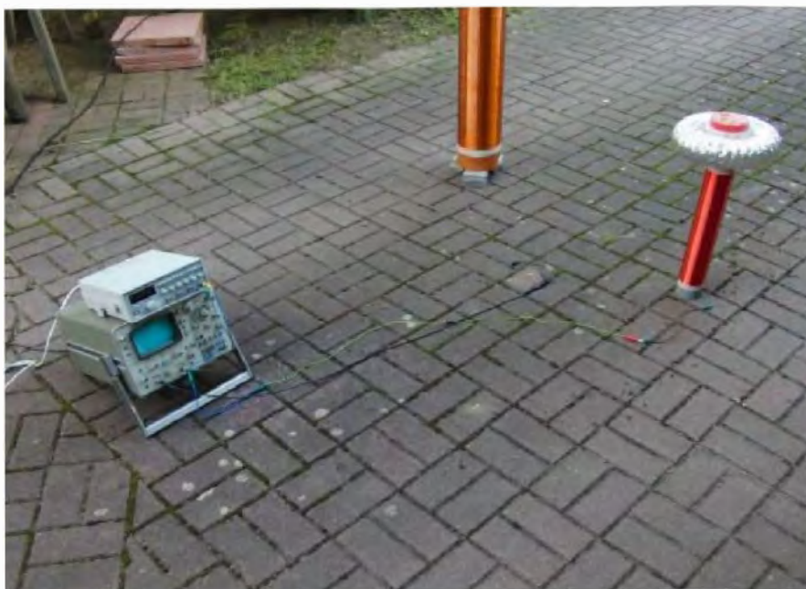
Figure 12: Determination of the resonant frequency of the secondary coil on the live object with sine wave generator and oscilloscope
