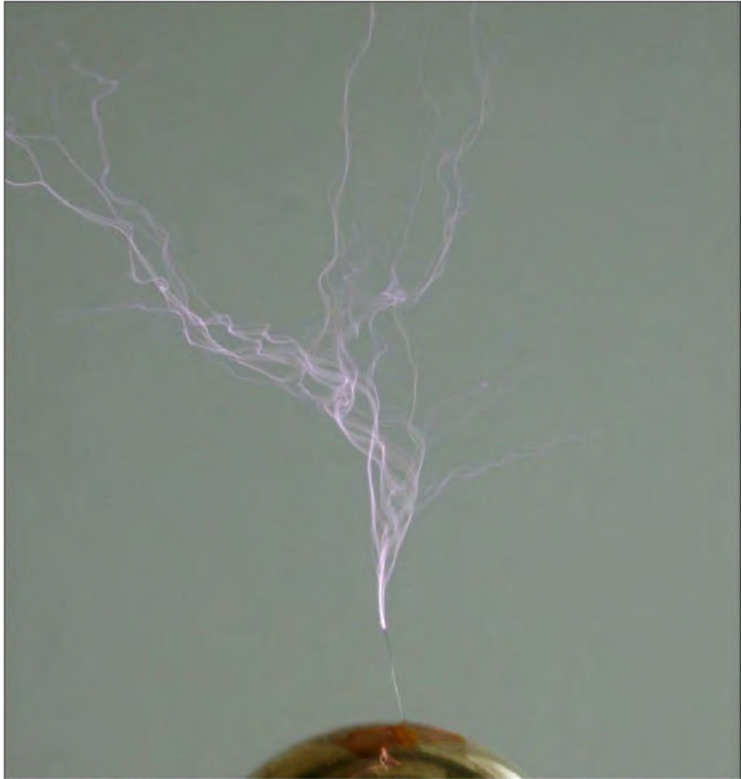
Detailed view of the streamers. The entrainment of the main channels located near the end of the wire by the air vortices occurring as a result of the heating can be clearly seen.
