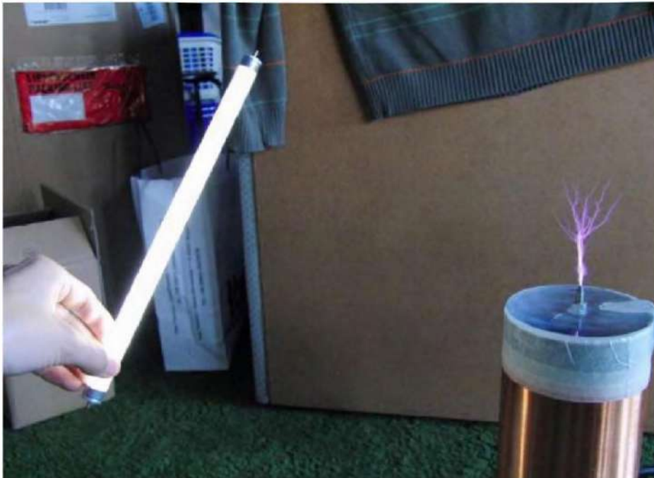
Figure 15: Detection of an RF field of a Tesla transformer
