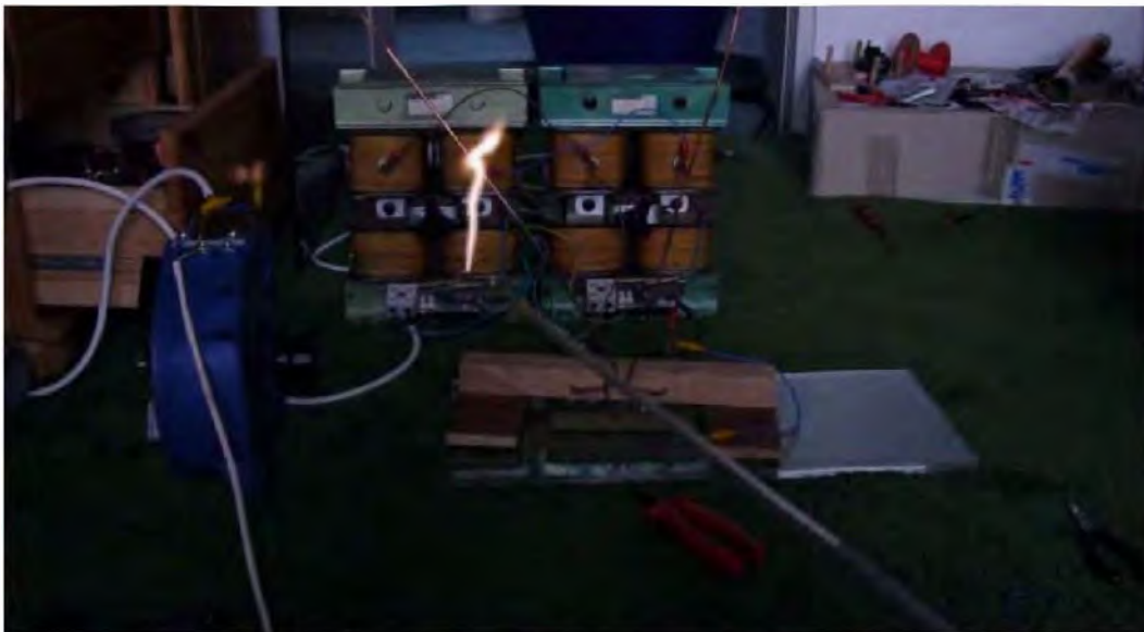
Figure 16: Arc with two neon transformers, temperature over 2500 degrees Celsius
