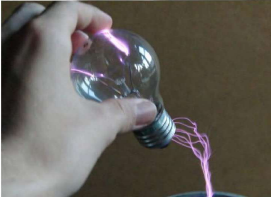
Figure 14: Plasma discharge in a light bulb
