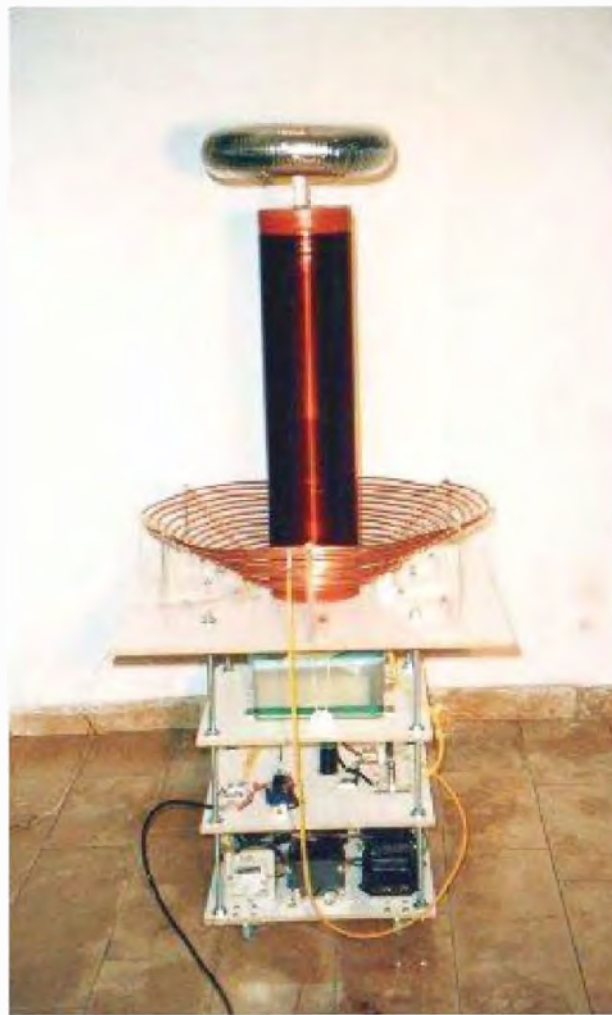
Figure 7: The finished Tesla coil shortly before commissioning
