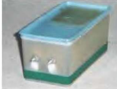
Figure 5: The finished high-voltage capacitor
