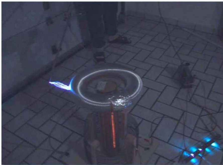
Figs. 18 and 19: Discharges against earth at different distances.
