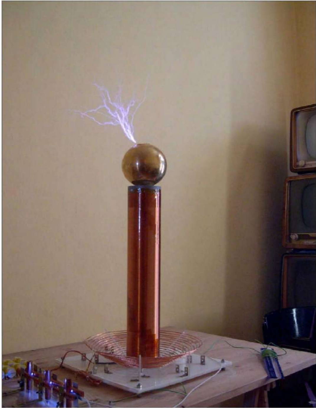
This image, taken with medium exposure time, comes very close to the actual impression. The discharges within the spark gap are also clearly visible.
