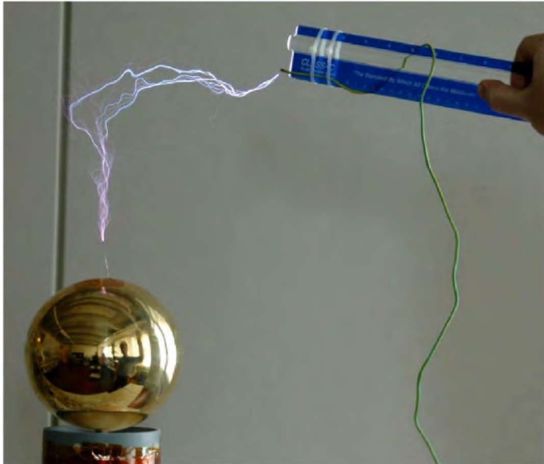
Here you can see the transition between the discharge in the form of streamers and the direct discharge to earth, as it occurs when the counter electrode approaches the head of the Tesla coil.
