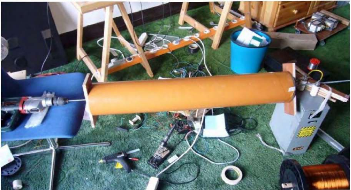
Figure 10: "Artful" winding machine for secondary coils, but it works!
