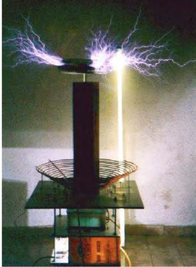
Fig. 9: The strong E -fields make the fluorescent tube glow
