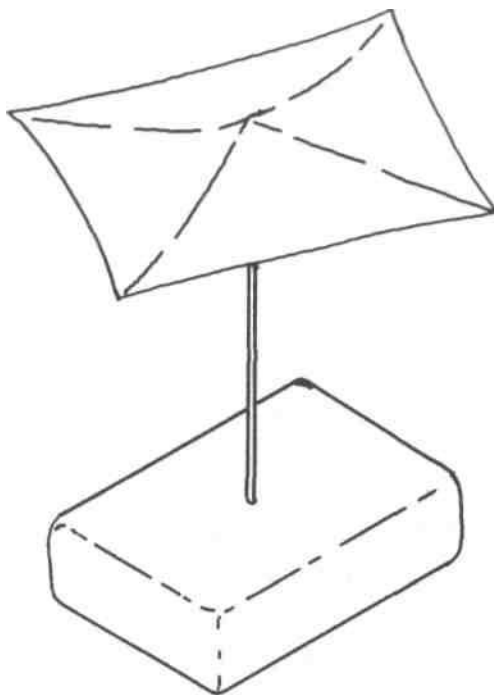
Figure 4-6: Drawing of the completed simple energy wheel. For ease of operation, you may want to set it atop an inverted water glass.
