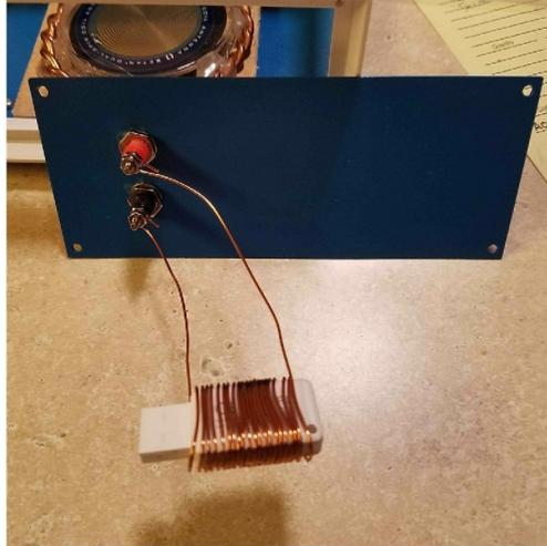
Reattach the front of the cabinet to the cabinet and bend the wire tails so the thumb-drive is centered over the Betar Coil. Here is a picture of the assembly before the tails are bent into place. You can also wait for this step until after you are done gluing inside of the cabinet. It is all a matter of how comfortable you are with tools.
