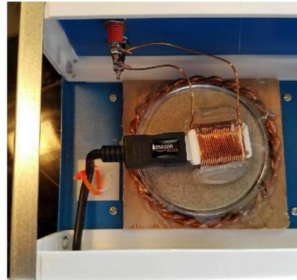
Drill a hole in the back of the cabinet large enough to fit the USB extension cable through. Connect the cable to the thumb-drive. Attach a strain relief to the cable so it doesn't move the drive when the cable is used. There are many different types of strain relief, choose one that will work for you.
